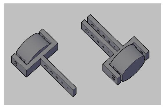
Figure 1. Design of shear box in AutoCAD 2010.
